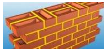
Alternating pattern of a solid wall
