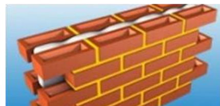
Regular brick pattern of a cavity wall
