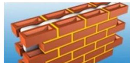
Regular brick pattern of a cavity wall
